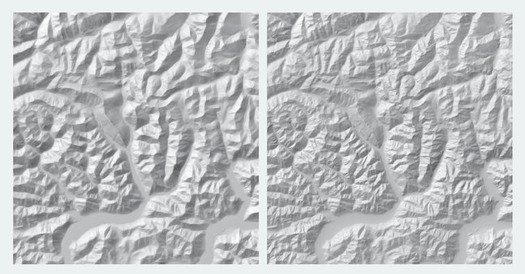
**Figure 12.** Normal median generalization (**left**) with exponential weights allows for very strong generalization of small features without blurring large features. In Pyramid Shader (**right**) the same terrain, with the same number of pyramid levels, cannot have its weights reduced further than what is shown here without visibly blurring the ridgelines and valley edges of large-scale features.
