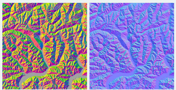
Figure 1. Two methods for displaying surface orientation. Left: an aspect-slope map. Right: a normal map.
