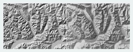
**Figure 7.** A standard analytical shaded relief (**left**) compared with a manual shaded relief by Imhof and Leuzinger (1963; shadedreliefarchive.com/Graubuenden\_SW.html; **right**). Despite deviating from what more physically accurate lighting would portray (or because it deviates from it), this style is better able to communicate a mental map of the relative significance of topographic features.
