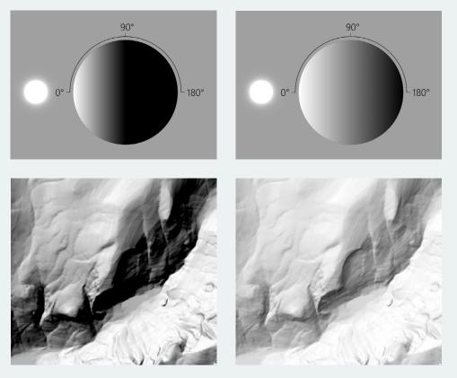
**Figure 6. Left:** Lambert shading will only illuminate surfaces that face toward the light source at least partially. **Right:** With the same lighting angle, soft hillshading preserves all the information in the surface, has a contrast profile that is less harsh, and requires less correction by the cartographer.
