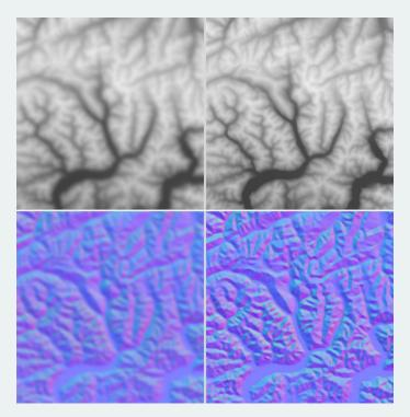
**Figure 10.** Comparison of Gaussian (**left**) and median (**right**) filters on an elevation raster (**top**) and a normal map (**bottom**). The normal median (lower right) has the best results in terms of eliminating noise while preserving scale-specific features of cartographic interest, and thus is used in the modified pyramid generalization algorithm.
