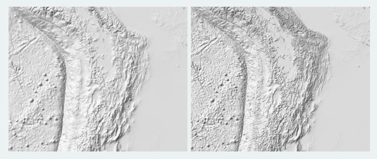
**Figure 8.** A comparison of an Andes hillshade based off generalized (**left**) and ungeneralized (**right**) elevation data. The area northeast of center is an especially good demonstration of how Lambert shading with an ungeneralized elevation raster can obscure large features.
