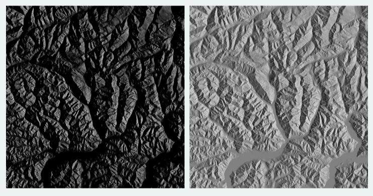
Figure 5. Left: A Lambert hillshade lit from the eastern horizon. **Right:** The normal map's x-band, or the same Lambert hillshade before the final step of the algorithm was performed.
