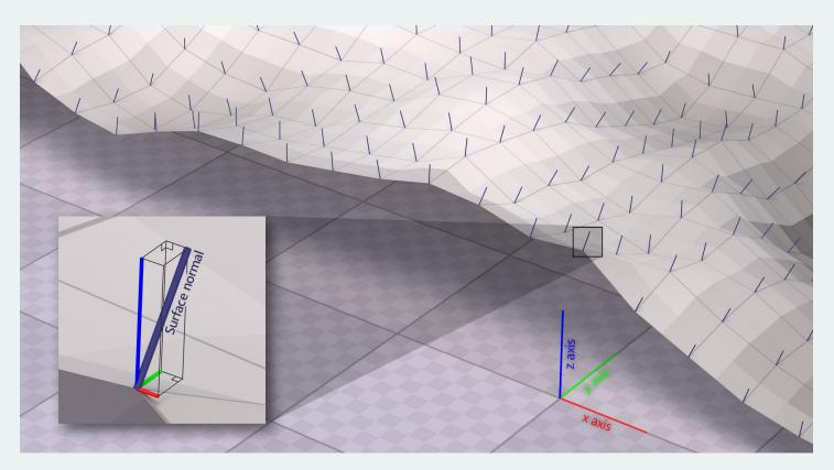
**Figure 2.** A 3D surface generated from an elevation raster. Each vertex represents the center of a raster cell, and the normals are drawn from these vertices, perpendicular to the average surface around them. **Inset:** the distances traveled along each axis by the normal are its components. This one travels a little bit to the east (positive x), a bit more to the north (positive y), and mostly upward (positive z).
