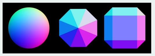
*Figure 14.* A reference for unit vector colors on, left to right, a sphere, a faceted cone with a slope of 45°, and a beveled cube.
