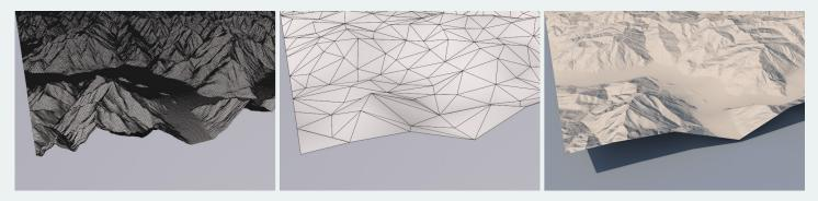
**Figure 4.** A dense mesh (**left**) may not draw fast enough for an interactive display, while a simplified version (**center**) may draw quickly but lack the desired detail. A normal map generated from the full-resolution mesh can be used to override the simplified geometry's normals during shading (**right**), giving the benefits of both.
