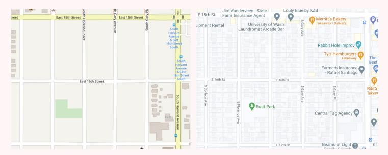
**Figure 15.** A comparison between maps from Mapbox (left) and Google (right) for a part of Tulsa, Oklahoma. The Mapbox map is missing most of the building footprints, as well as property boundaries.
