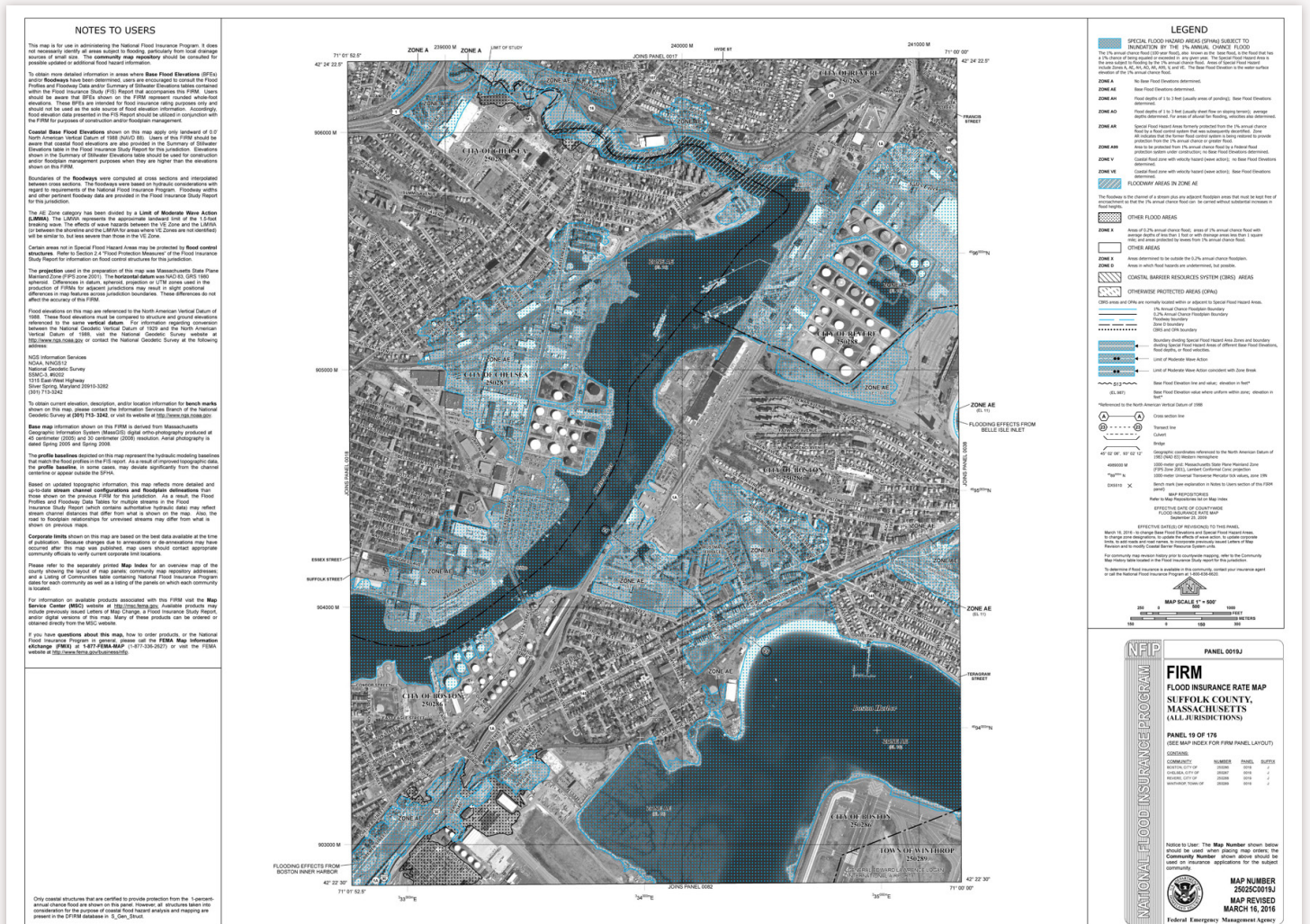
Figure 2. A FIRM depicting flood risk for part of Suffolk County, Massachusetts. Orthoimagery is included in this FIRM but is not standard across all FIRMs, nor is any particular color scheme. Obtained from msc.fema.gov/portal .
