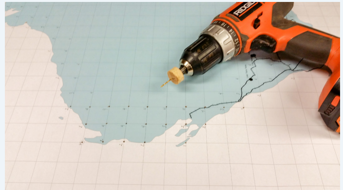
Figure 1. Map showing labeled intersections and ⅛-inch (0.32 cm) drill setup for starter points.
