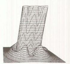
The H-CO<sub>2</sub> interaction is highly repulsive (an energy of at least 110 kJ/mole) everywhere (the "foothills" before the tall mountains except along a line perpendicular to the OCO axis at the C atom. Here there is a small plateau with an energy of 54 kJ/mole, and beyond this a well or valley corresponding to stable H-CO<sub>2</sub> where H is attached to the C atom.
