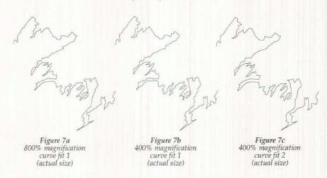
Figure 7: Effects on line character of variations in magnification level and curve fit setting.
