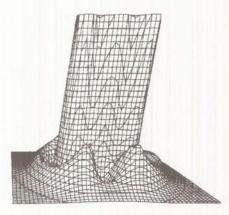
The H-CO<sub>2</sub> interaction is highly repulsive (an energy of at least 110 kJ/mole) everywhere (the "foothills" before the tall mountains except along a line perpendicular to the OCO axis at the C atom. Here there is a small plateau with an energy of 54 kJ/mole, and beyond this a well or valley corresponding to stable H-CO<sub>2</sub> where H is attached to the C atom.
