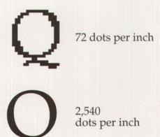
Figure 2: The quality of imagesetter output depends largely on resolution
