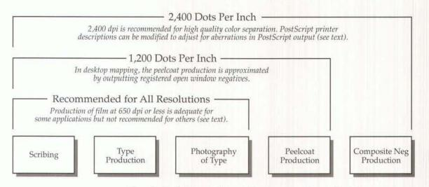
Figure 3: Acceptable imagesetter resolutions for cartographic production tasks
