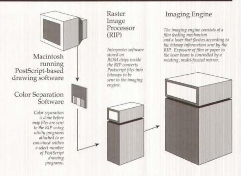
Figure 1: The imagesetter as part of the complete desktop mapping system
