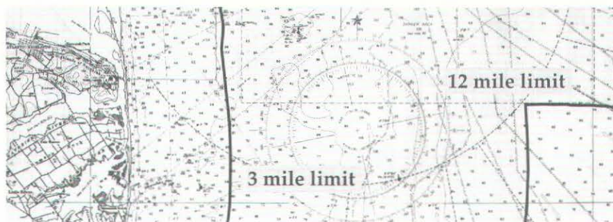
Figure 1: 3- and 12-nautical mile limits on a black-and-white 50 percent reduction nautical chart. (Lines have been widened and darkened for illustration purposes.)
