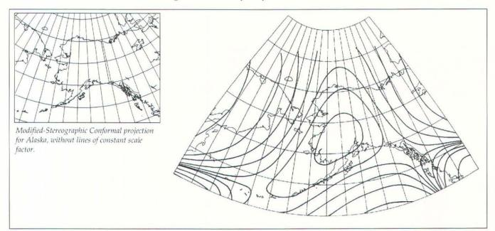
Figure 18. Modified-Stereographic Conformal projection for Alaska, with lines of constant scale factor.
