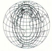
Figure 24. Ginzburg Pseudoazimuthal projection for Atlantic Ocean, with oval lines of constant maximum angular distortion (5°, 10°, 15°, 20°).
