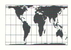
Figure 2. Gall Orthographic (Cylindrical Equal-Area) projection.
