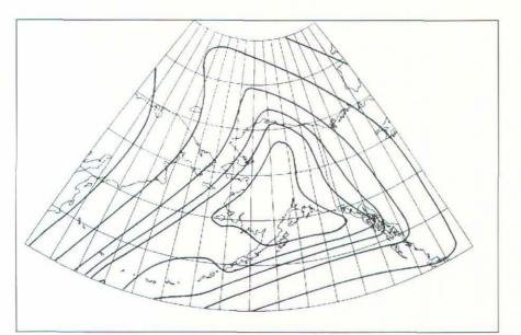
Figure 22. Low-Error Equal-Area projection for Alaska, with lines of constant max. scale factor.
