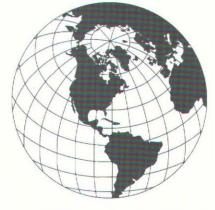
Figure 25. Oblique Lambert Azimuthal Equal-Area projection for hemisphere centered on Washington, D.C.
