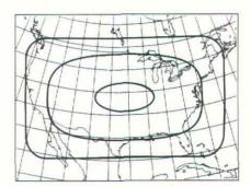
Figure 19. Modified-Stereographic Conformal projection for 48 United States, with lines of constant scale factor (.99, 1.00, 1.011).
