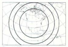
Figure 16. Oblique Stereographic projection, with lines of constant scale factor (1.1, 1.2, 1.3).
