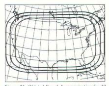
Figure 21. Oblated Equal-Area projection for 48 United States, with lines of constant max. scale factor (1.01, 1.0125, 1.015).
