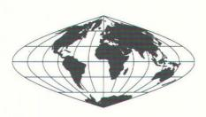
Figure 6. Sinusoidal projection.
