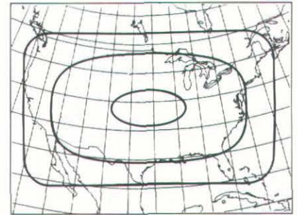
Figure 19. Modified-Stereographic Conformal projection for 48 United States, with lines of constant scale factor (0.99, 1.00, 1.011).
