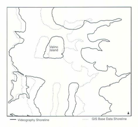
Figure 2. Comparison of Camera Lens Distortion Effect on Shoreline
