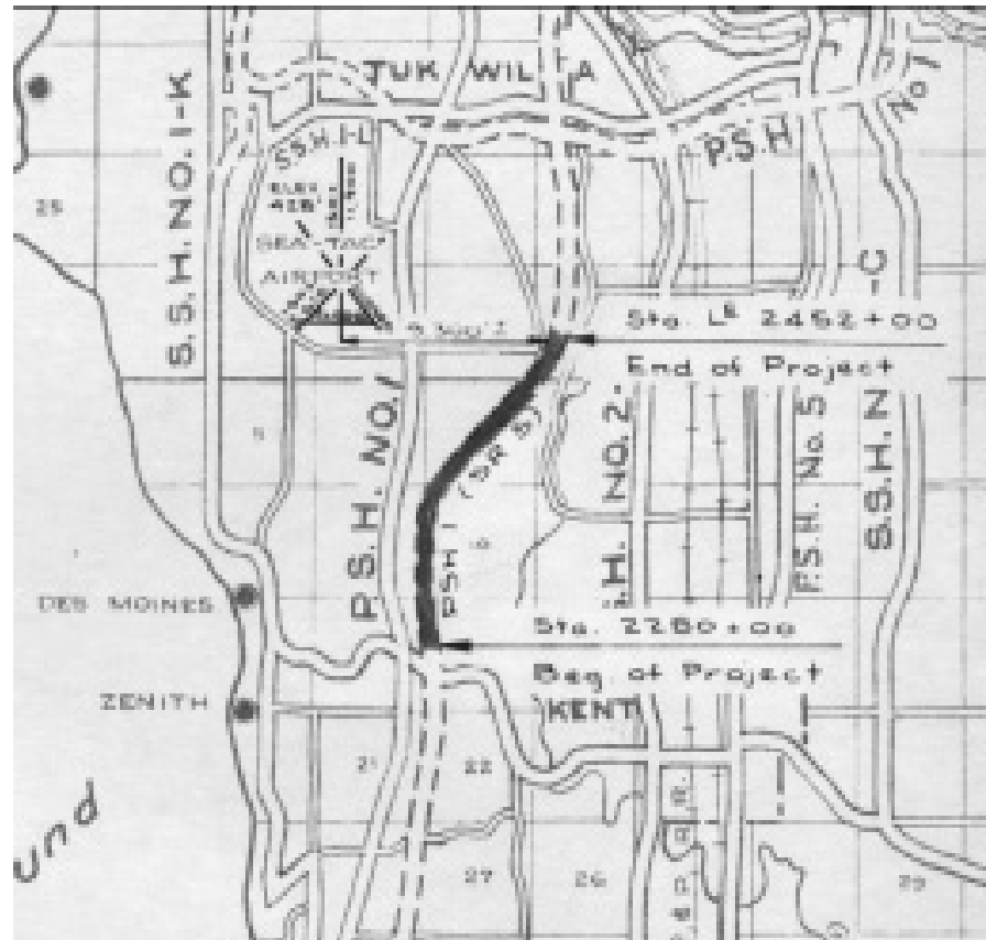
Map 4. Open-cased road maps provided the base for manually interpolating the location of information by route and milepost. Here, a construction project is plotted and labeled with “stationing,” a kind of linear reference system used by highway engineers. (ca. 1970. Courtesy of Washington State Department of Transportation)
