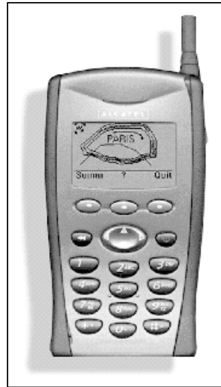
Figure 3. An example of an internet based mapping service, combined with real-time traffic information, and delivered to a WAP enabled mobile phone.
