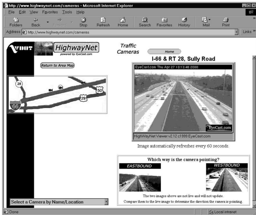
Figure 3. Webcam (right) shares the screen with a detailed index-map excerpt (left) on which camera-like icons show webcam locations. Faint circle surrounding the center icon marks the camera's location. Pair of example views below the webcam image helps the viewer identify direction in which the camera is pointing.
