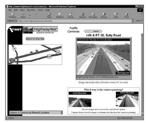
Figure 3. Webcam (right) shares the screen with a detailed index-map excerpt (left) on which cameralike icons show webcam locations. Faint circle surrounding the center icon marks the camera's location. Pair of example views below the webcam image helps the viewer identify direction in which the camera is pointing.
