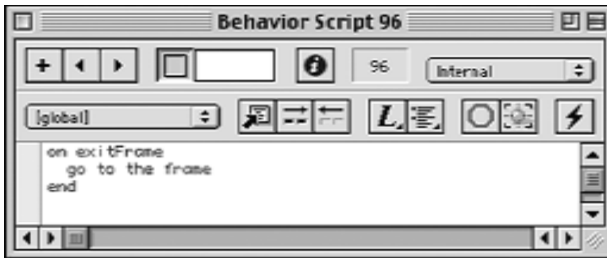
Figure 2. This script is associated with a specific frame and is accessed via Modify > Frame > Script . The script is called when the movie plays through that frame (exits the frame) and keeps the movie on that frame (keeps cycling through that frame).
