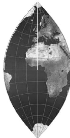
Parallels should meet meridians at right angles so there are no links in the seams between gores. But if parallels curve to meet the meridians at right angles, then the distance between parallels cannot remain constant.
