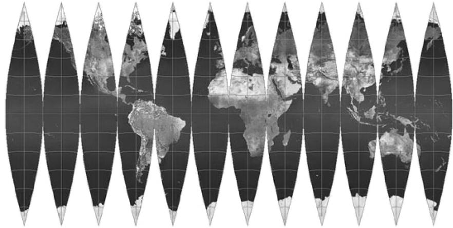
In order for a projection to be interrupted easily in a general way, spacing of meridians must be constant along the equator. Most of those projections are pseudocylindrical. Pseudocylindrical projections have straight parallels, so they do not meet the meridians at right angles. Hence, pseudocylindrical projections are not suitable for globe gores. Projections suitable for gores are rare.
