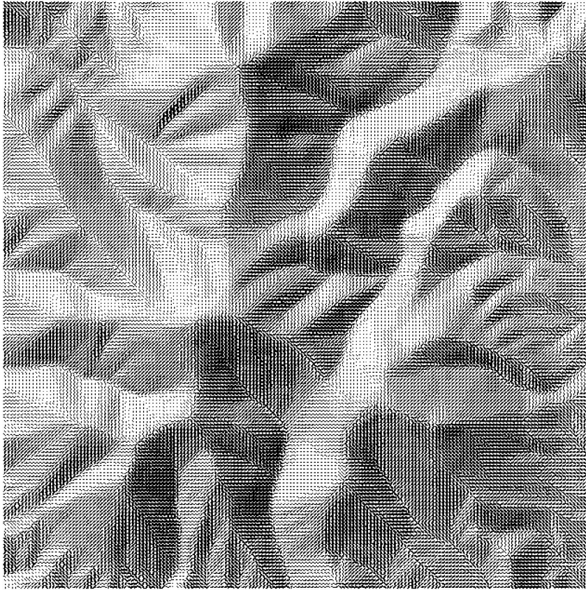
Figure 17. The same hillshaded map in Figure 15 dithered with the halftone patterns from Figure 9 oriented in the aspect direction.
