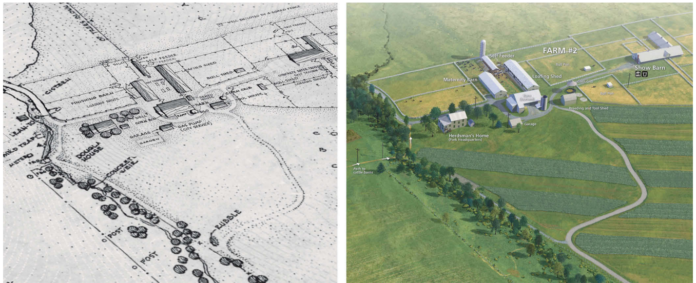
Figure 5. A portion of Eisenhower National Historic Site, Pennsylvania. (left) A plan map draped on a DEM and viewed obliquely in Bryce. The park approved this view as the basis for final production. (right) The final bird's-eye view. Art at right by Chris Casady.
