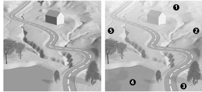
Figure 20. (left) A simple scene rendered without environmental special effects. (right) The same scene with exaggerated special effects, which include (1) background haze; (2) pale yellow illumination coming from the lower right; (3) soft cast shadows; (4) reflective water surface; and, (5) secondary blue light coming from the left. Environmental special effects come at a price; the scene on the left took 12 minutes to render compared to 2 hours and 18 minutes for the scene on the right. (see page 105 for full color version)
