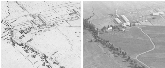
Figure 5. A portion of Eisenhower National Historic Site, Pennsylvania. (left) A plan map draped on a DEM and viewed obliquely in Bryce. The park approved this view as the basis for final production. (right) The final bird's-eye view. Art at right by Chris Casady. (see page 97 for full color version)
