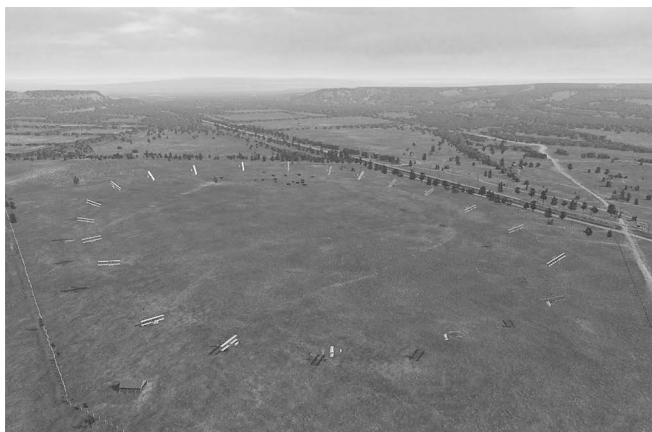
Figure 12. This scene shows the counter-clockwise flight of the Wright Flyer in 1908 over the Huffman Prairie Flying Field, Dayton, Ohio. The foundation of the scene is a custom DEM at 3-meter resolution derived from contour lines processed in ArcGIS software. A second hand-made DEM with a bumpy dark-green texture extrudes upwards through the surface of the first DEM to depict background trees. Art by Chris Casady. (see page 100 for full color version)
