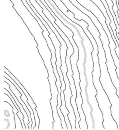
Figure 7. Jagged contour lines resulting from corduroy effect on DEM data.
