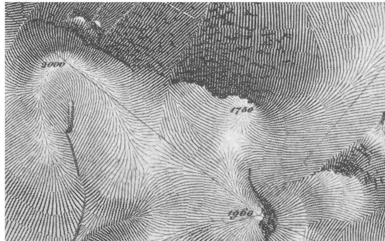
b) Terrain rendering using slope hachuring
