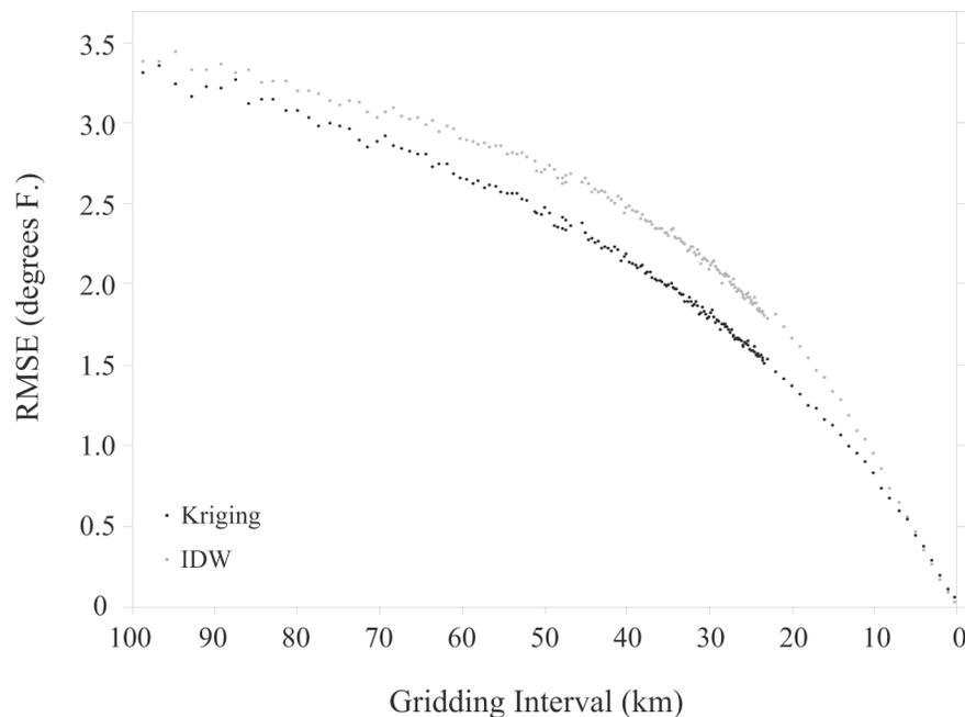
Figure 2. Scatter plot showing relationship between RMSE and gridding interval for kriging and IDW.
