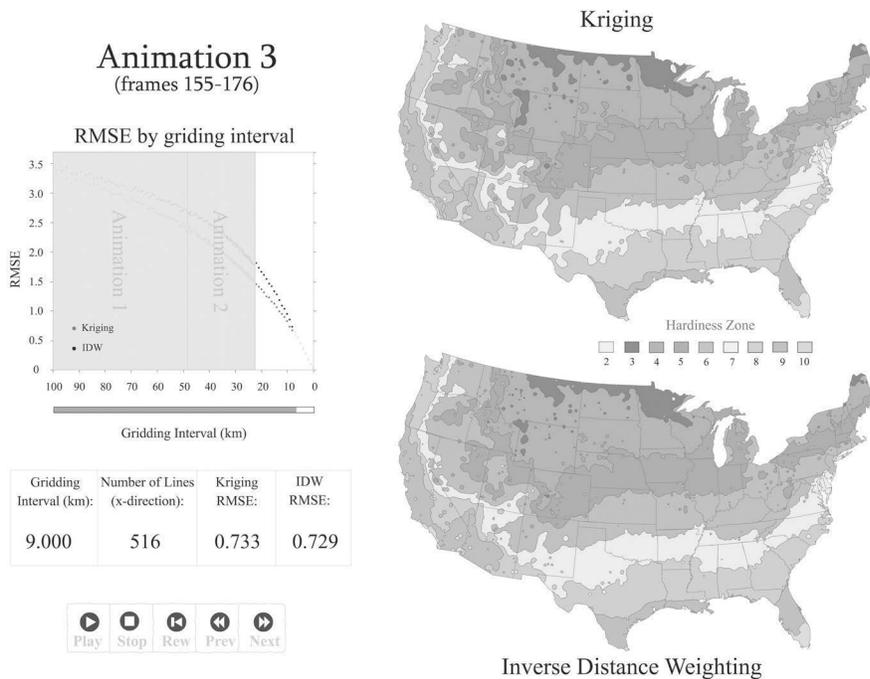
Figure 8. Screen capture of frame 169 of Animation 3 showing the difference in patterning for kriging and IDW when RMSE values are nearly identical. (see page 74 for color version)
