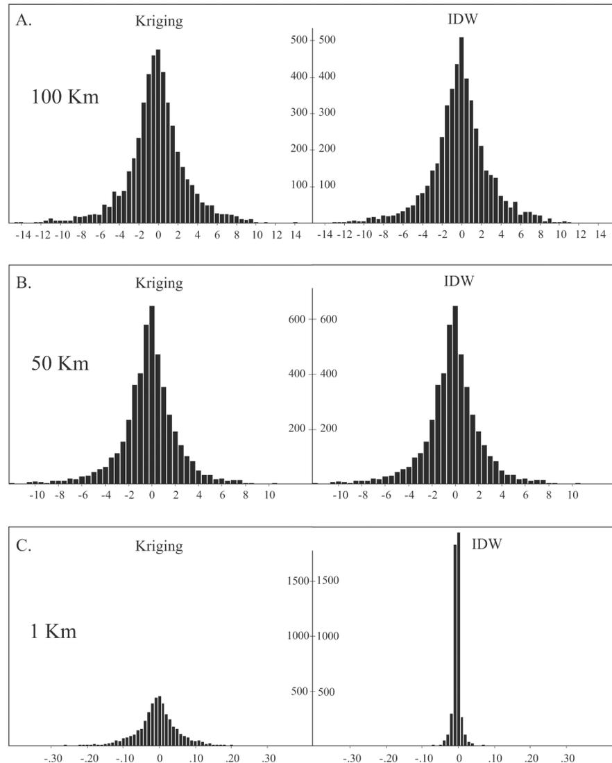
Figure 3. Distribution of the residuals (difference between predicted and observed values for each of the 4,799 weather stations) used for calculating RMSE for selected gridding intervals. a) Gridding interval is 100km. b) Gridding interval is 50 km. c) Gridding interval is 1 km.
