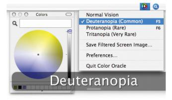
Figure 1. Screenshot of Color Oracle on Mac OS X simulating deuteranopia on a color picker wheel.
