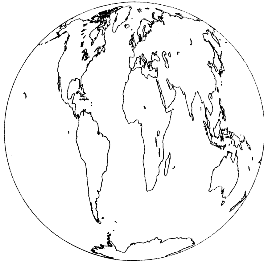
Figure 9. Mollweide's equal area projection affinely modified to fit in a circle. The equal area property is retained.
