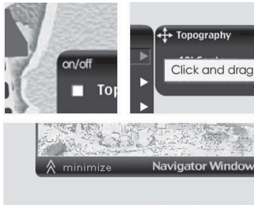
Figure 11. Redesigns for the layer visibility button (top-left), the tear-away menu button (top-right), and the minimize window button (bottom) added words to explain the function of the widget and sometimes did away with the vague icon altogether. Tool tips (top-right, in yellow) also appear after pausing over a widget for one second to further prompt the user about the widget’s function. (see page 93 for color version)
