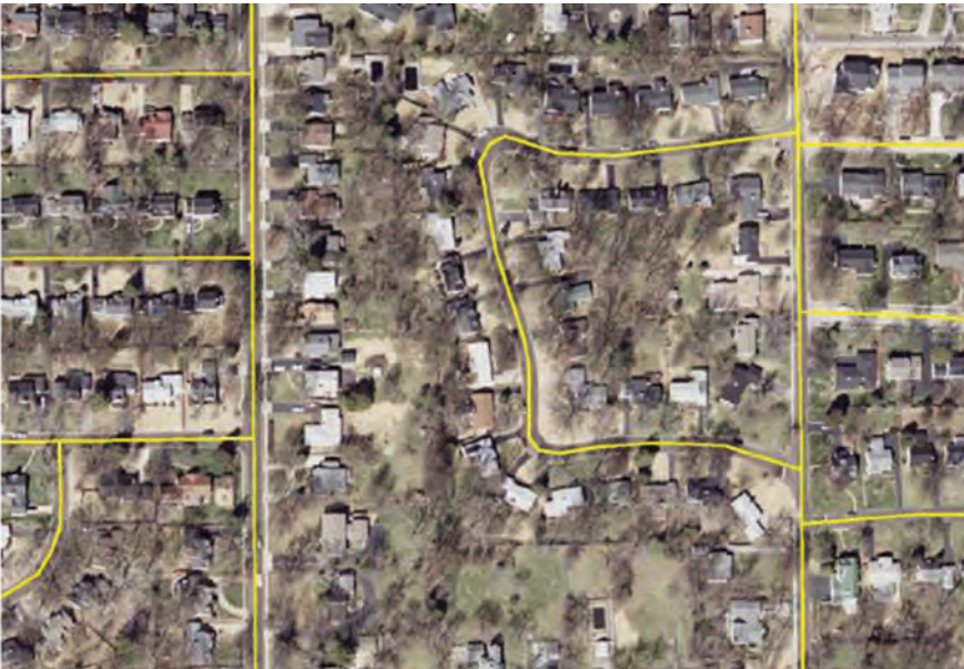
Figure 6. A vector transportation dataset was manually edited to match the orthoimages. The display of the manually edited data over the orthoimage became the standard against which qualitative evaluations were based.
