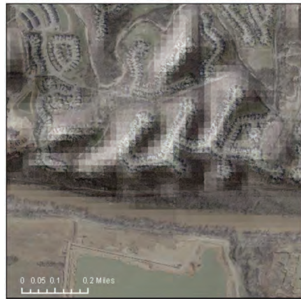
Figure 3. An orthographic image with 0.33 m pixel overlaid with elevation data with 30 m pixels.
