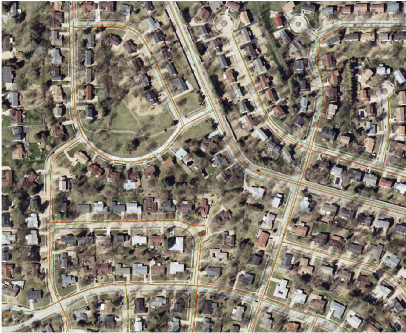
Figure 7. MODOT and orthoimage integration after implementation of the automated procedure showing improvement in alignment for integration (red: MODOT; green: automatically processed roads).
