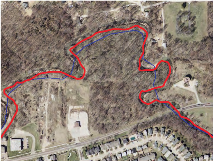
Figure 5. Example of generalization problem for data integration. The blue line is the generalized stream as represented in the Census TIGER data, which was developed from the USGS 1:100,000-scale topographic map; the red line represents the true stream course without generalization.
