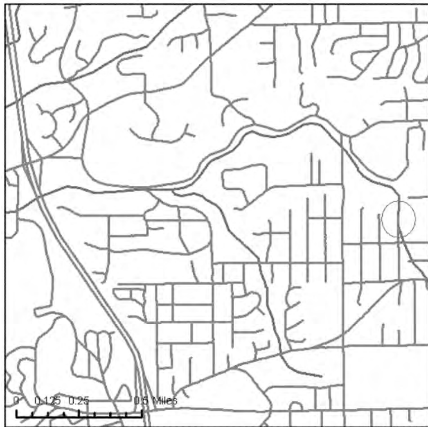
Figure 4. Vector data for roads (red) and streams (blue) overlaid for the same areas. Note the area in the purple circle where the stream follows the road centerline. (see page 60 for color version)
