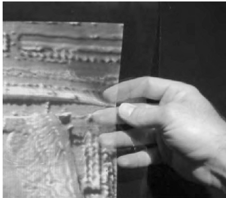
Figure 2. Digital holograms recorded on photopolymer film.
