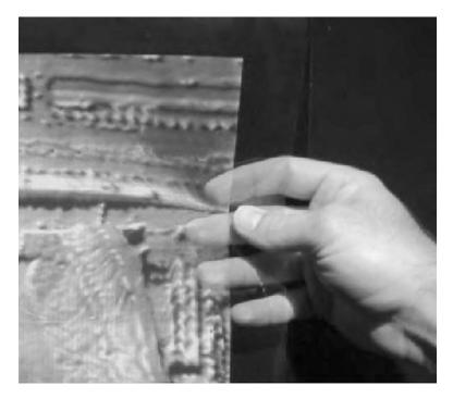
Figure 2. Digital holograms recorded on photopolymer film.
