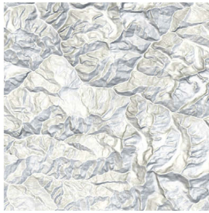
Figure 3. Oblique relief shading combined with slope shading with yellow highlights and blue shadows.
