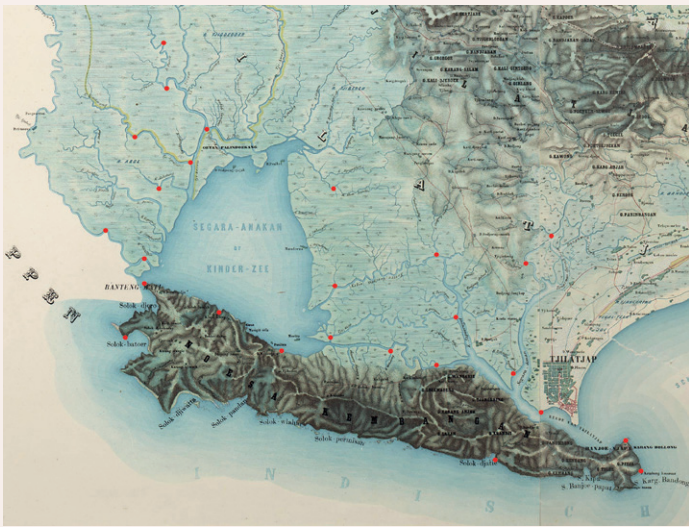
Figure 5. Section of the Topographische Kaart van de Residentie Banjoemaas, based on surveys carried out between 1857 and 1860. Original scale: 1:100,000. Retrieved from the Netherlands Royal Tropical Institute (KIT). The red points represent the ground control points used for georectification.
