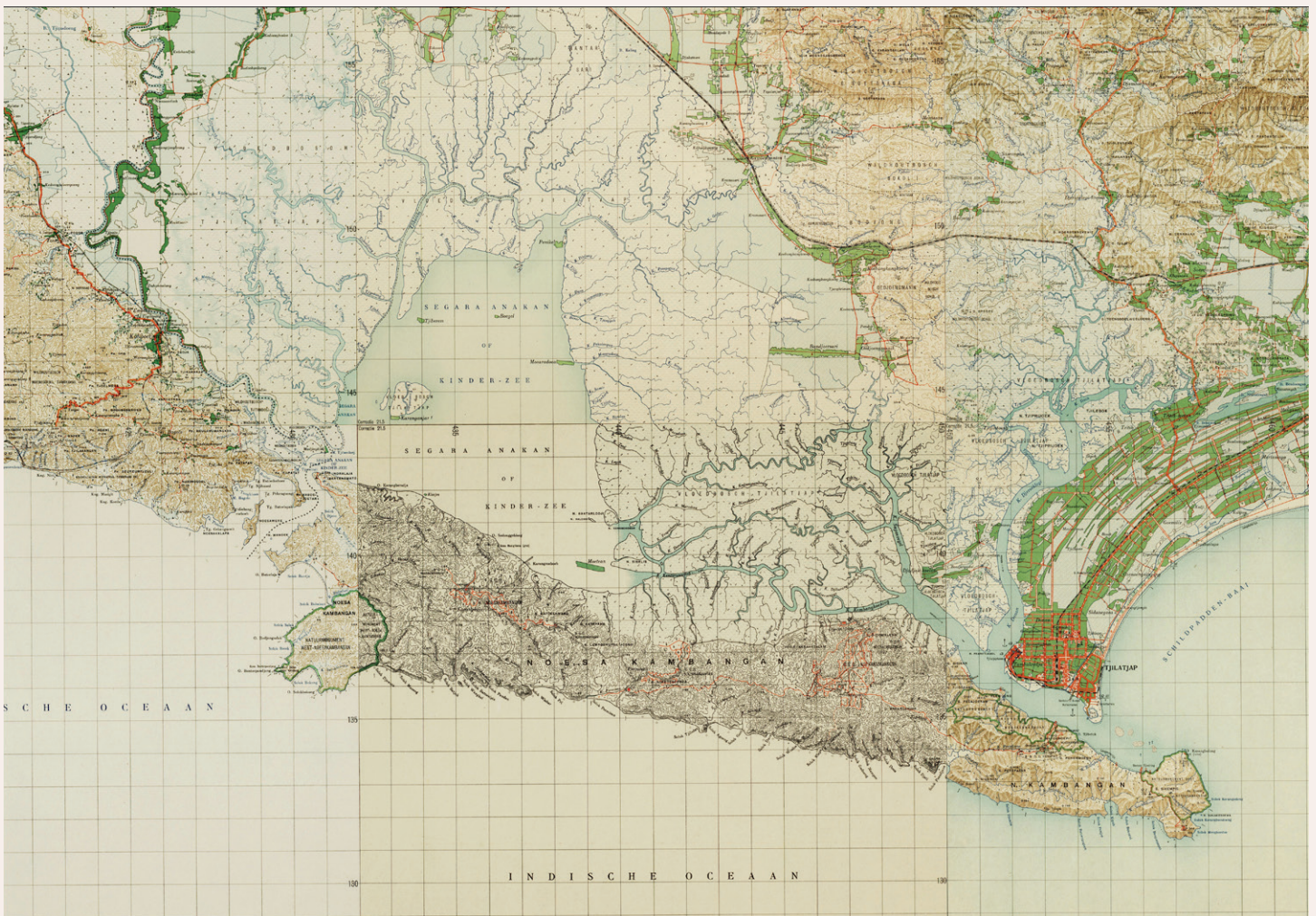
Figure 7. Topographic map of Java, Middle and West Java, produced by TDNI, mainly based on surveys carried out between 1924 and 1926. Compilation of sections of map sheets 42/XLI D, 43/XLI C, 43/XLI D, 42/XLII B, 43/XLII A, 43/XLI D. Original scale: 1:50,000. Retrieved from KIT.
