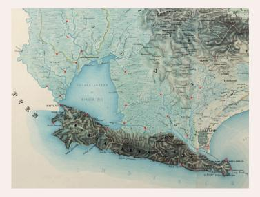
*Figure 5.* Section of the Topographische Kaart van de Residentie Banjoemaas, based on surveys carried out between 1857 and 1860. Original scale: 1:100,000. Retrieved from the Netherlands Royal Tropical Institute (KIT). The red points represent the ground control points used for georectification.
