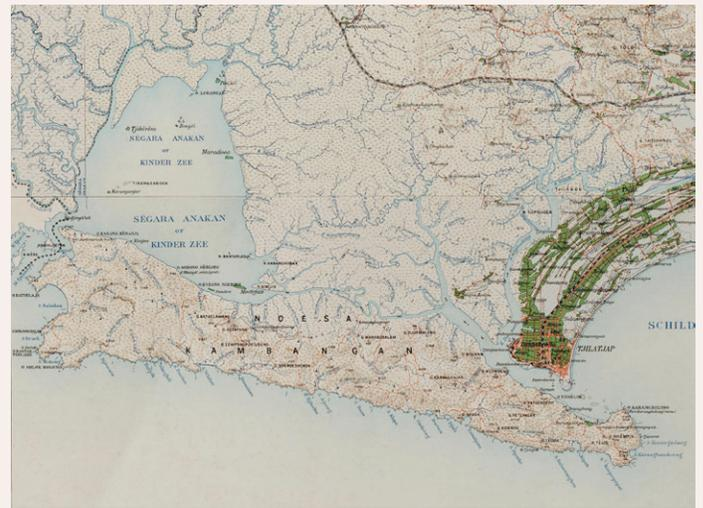
**Figure 6.** Topographic map of Java, Residency Banjoemas, produced by the Topographical Service in the Netherlands East Indies (TDNI), based on surveys carried out between 1897 and 1901. Compilation of sections of map sheets III, IV, VII, and VIII. Original scale: 1:100,000. Retrieved from KIT.
