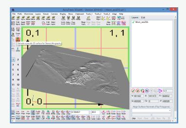
Figure 8. To avoid a wafer-thin model, extrude your surface.
