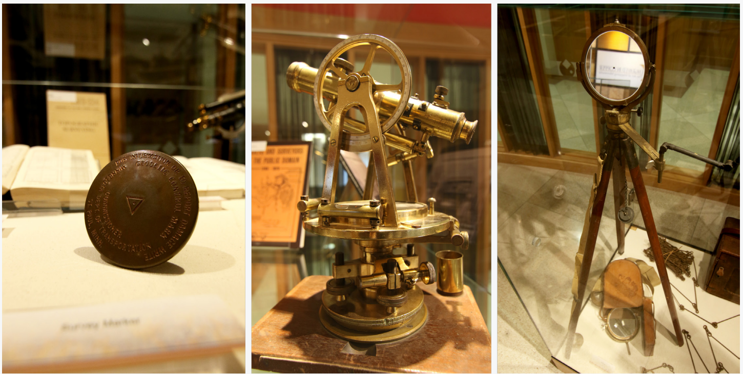
Figure 5. From left to right: survey marker, transit, and heliotrope.
