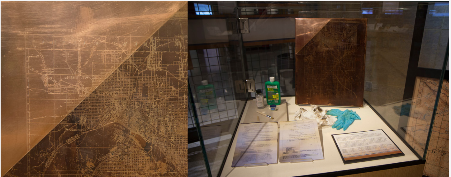
Figure 2. Left: detail of a copper plate showing before and after cleaning. Right: display case highlighting the cleaning process.
