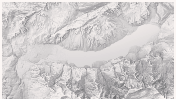
Figure 6. Ambient occlusion darkening a lake and a valley bottom (top); ambient occlusion reduced in flat areas (bottom). Scan radius r = 200 pixels, aperture angle \alpha = 200^\circ . Klöntalersee, Switzerland, swissALTI3D elevation model by swisstopo downsampled to a 10-meter resolution.
