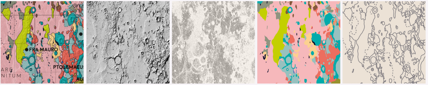
Figure 8. A finished section of the combined map (far left), as well as some of the individual pieces including the hillshade, slope, geologic unit colors, and geologic structures.
