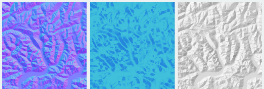
Figure 13. The dot product between a generalized normal map (left) and a light vector raster derived from one of the pyramid levels used to make that normal map (middle) is a soft hillshade with a variable light source (right). Note that the brightest parts of the hillshade are where the normal map and light vector colors are most similar. In the light vector raster, cyan corresponds to standard lighting from the northwest and blue corresponds to lighting from the southwest, both elevated 45°.
