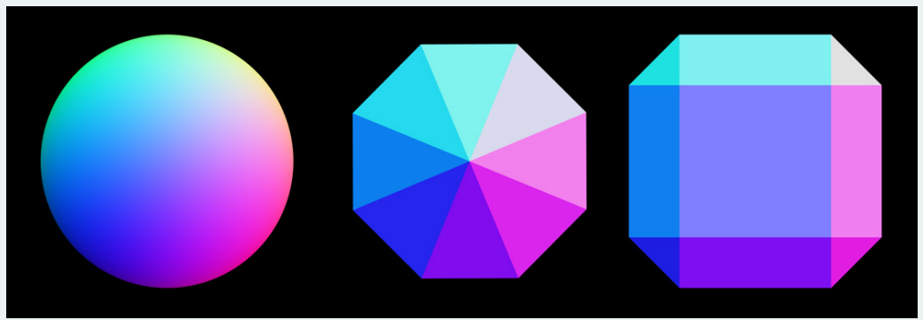
Figure 14. A reference for unit vector colors on, left to right, a sphere, a faceted cone with a slope of 45°, and a beveled cube.
